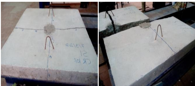
(a) Top Surface (b) Complete Failure Figure 8. The crumb rubber concrete slab (CR 10%)
