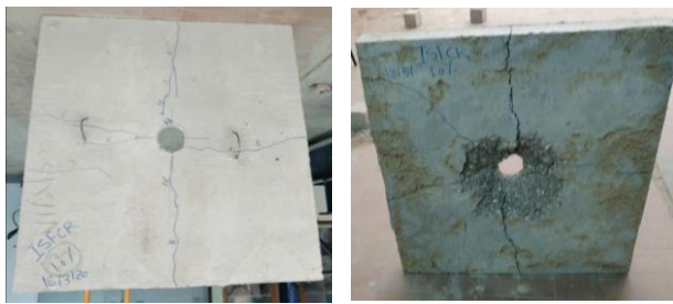
(a) (b) Figure 14. ISFCR 1.0% (a) Top surface; (b) Bottom surface
